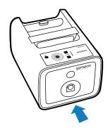
2 Check that the air intake areas on the front and underneath SIMEOX are not blocked. Air must circulate freely all around and under the device; Connect the power cable to SIMEOX.
