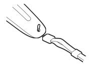
1) Slide the cord into the hole of the remote control
