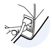
4 Turn on the device by setting the power switch on the back of the device to position "1". The light of the "standby/on" button of the control pad turns yelloworange. Your SIMEOX is in "standby" mode and ready to be used.
